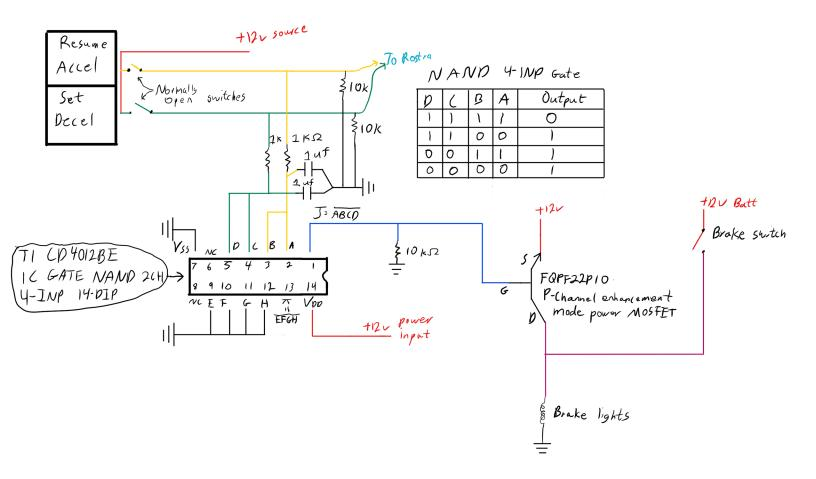
It is a reasonable assumption that the Rostra cruise unit has internal pull down resistors on the Yellow and Green input sense wires. I have added my own to be safe.
